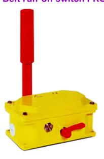
Robust belt run-off switch. Two switching elements are actuated by different cams on the shaft.
