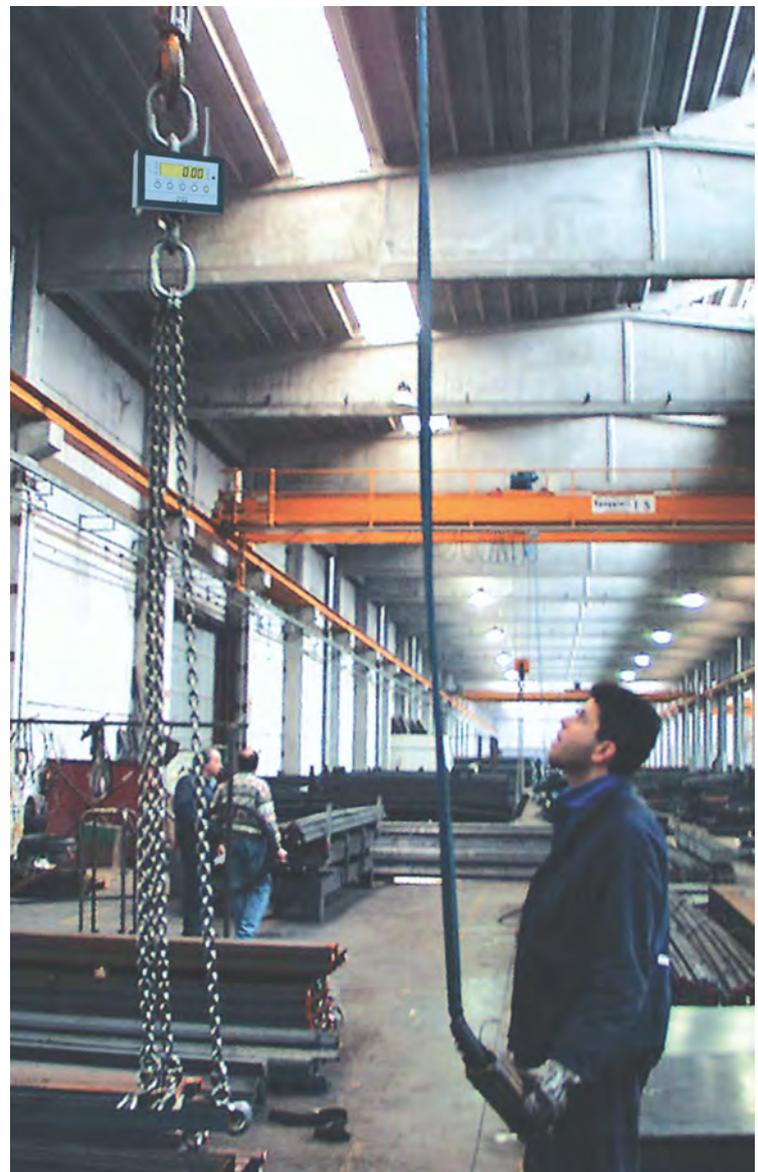
For weighing by way of legal transaction, OIML approved crane scales are available, optional with integrated alibi memory. We offer versions with ATEX approval for the use in hazardous areas, too.
