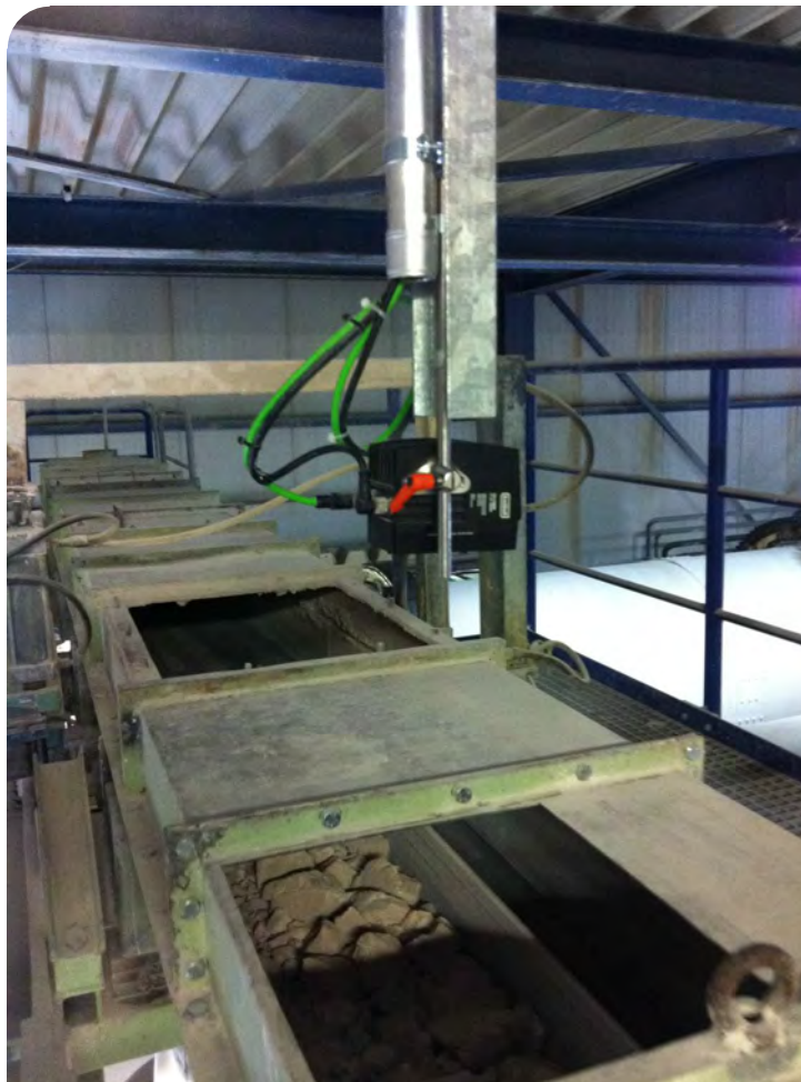
Limestone measurement on a vibrating conveyor
